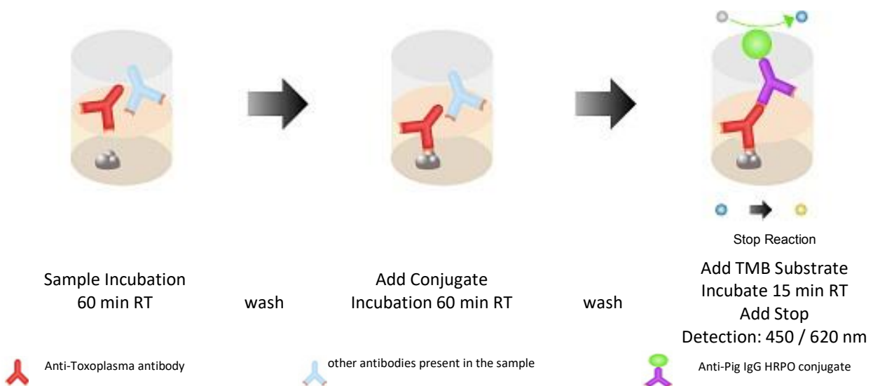
Figure 1: Schematic diagram of the procedural steps of the ELISA reaction. The ELISA kit from Prionics and was performed as described in the kit instructions. The absorbance of each well was measured at 450 nm with a reference measurement at 620 nm.
